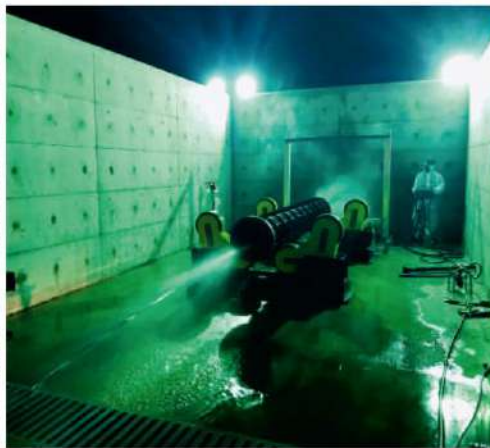
Inside and outside high pressure cleaning of bundles with proper equipment in the least possible time.
